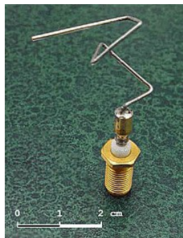
Figure 12: Evolved antenna (Source: https://en.wikipedia.org/wiki/Evolved_antenna ) via evolutionary algorithms; used on a 2006 NASA spacecraft.
