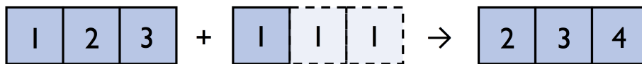
Figure F.4: An illustration of broadcasting showing the addition of a single number to every element in an array.
